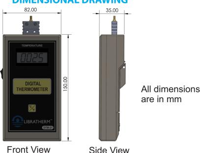
Note: Dimension of DTM-21, DTM-22 & HTM-22 are same
